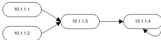
Fig. 1. Intrusion detection alarms from Table 1 as a directed graph
